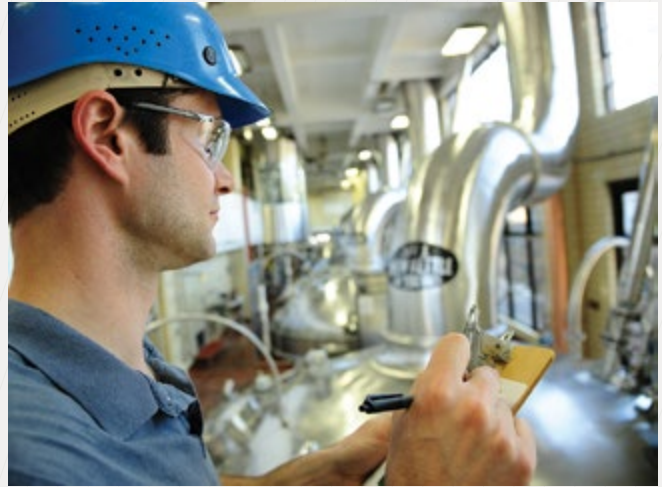
Dan Pearson, brewing optimization engineer, monitors and optimizes the brew kettle clean-in-place sequence to reduce water usage.
