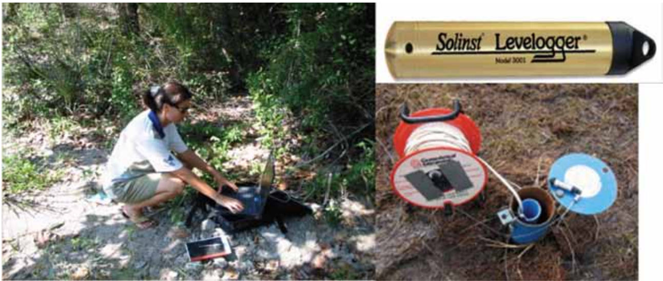
Figure 20: A data logger such as this Solinst logger is suspended in a borehole at a fixed depth to record changes in the groundwater level. This level should be verified with a dip meter. Data may be downloaded at the borehole directly onto a lap top, or it may be downloaded remotely and accessed via the internet.
